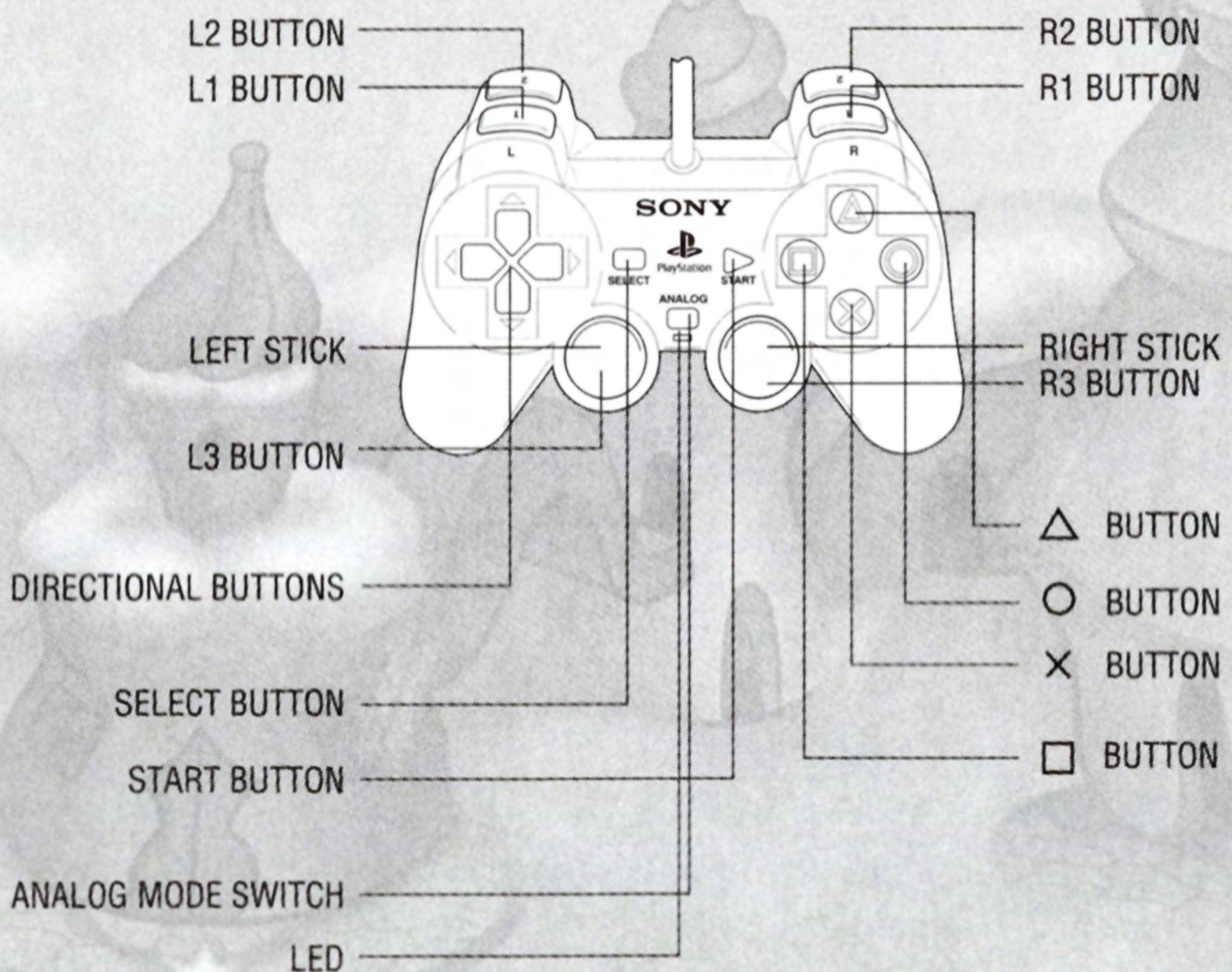
**Note:** The Left Stick of the DUALSHOCK™ analog controller is functional only in ANALOG mode when the ANALOG mode switch LED is ON (lit). Press the ANALOG mode switch to toggle the LED ON/OFF.
